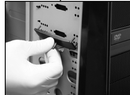
Attach the screw less bracket matching the 5.25" holes
