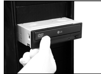
Insert the 5.25" Device through the opening
