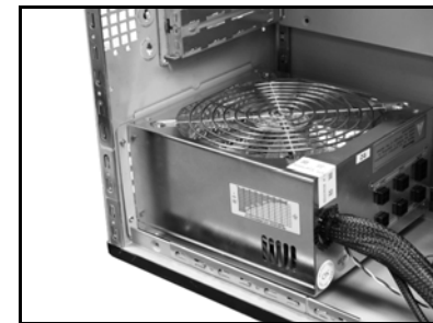
PSU at the bottom of the chassis
