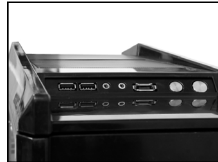
USB, Audio ports, E-SATA, Reset, and Power buttons
