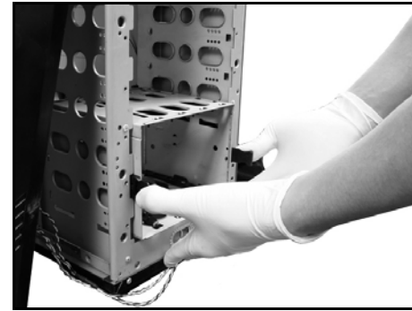
Push the tabs to remove the cage
