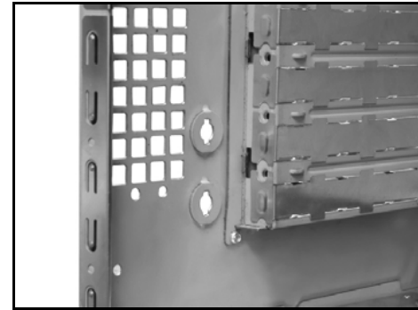
Water tubes can be routed in from behind the case.
