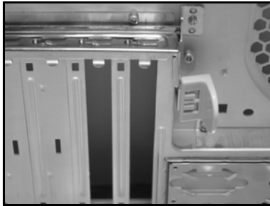
Fastener Figure. Push down here to lock the fastener
