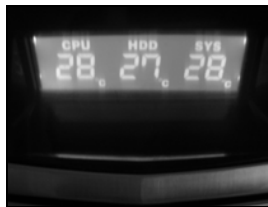
From Left to Right. CPU, Hard Drive, System Temperature Display
