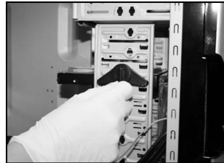
Screwless for 3.5" internal device ( ie Hard drives )
