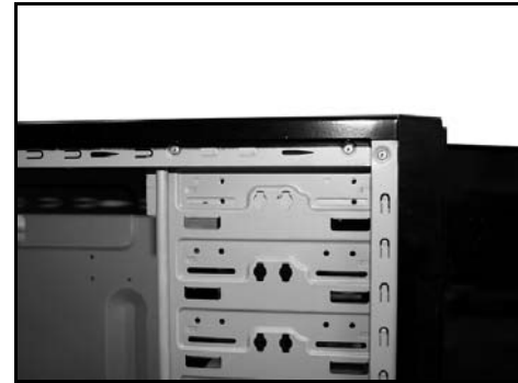
Matching the holes to the 5.25" device.
