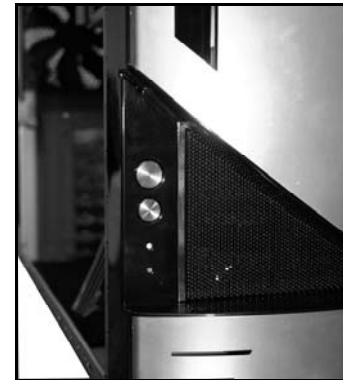
The front panel Power, Reset, Power LED, and HDD LED locations
