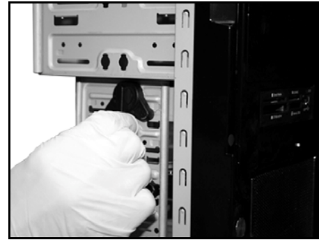
Screwless for 3.5" external device.
