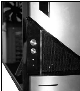
The front panel Power, Reset, Power LED, and HDD LED locations
