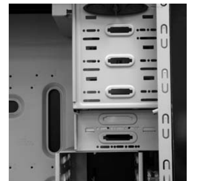
Matching the holes to the 3.5" bays
